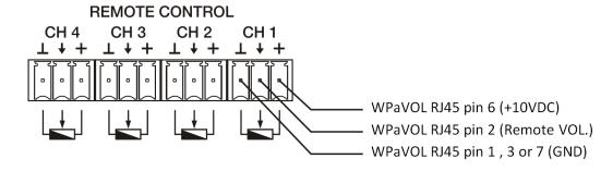
Connection of WPaVOL to remote-control ports
